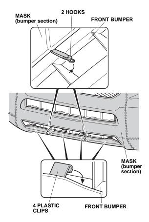
17. Attach six hooks to the bottom inside edge of the front bumper as shown.
