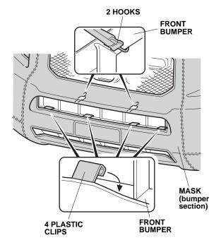
16. Attach four plastic clips and two hooks to the bottom inside edge of the front bumper as shown.
